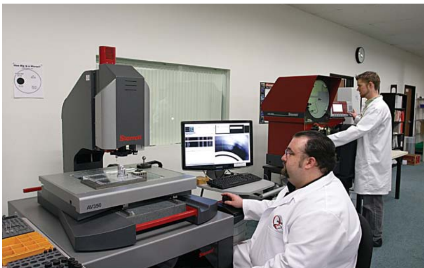
Lab manager John Michael Lyons uses a Starrett AV350 multisensor CMM. Jason Sommers works at an optical comparator.
