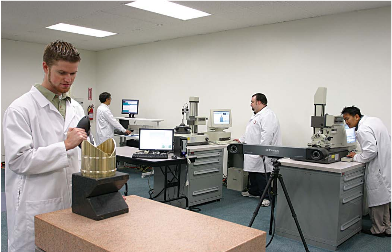
Jason Sommers, foreground, uses a Creaform wireless CMM to check an aerospace part. Yoichi Mizutani, quality manager, far left, measures a medical part using the optical probe on a coordinate measuring machine. Jack Nguyen, right rear, uses a contour tracer to measure a 2D profile. Middle rear is John Lyons using a form tester to check the cylindricity of a valve body.
