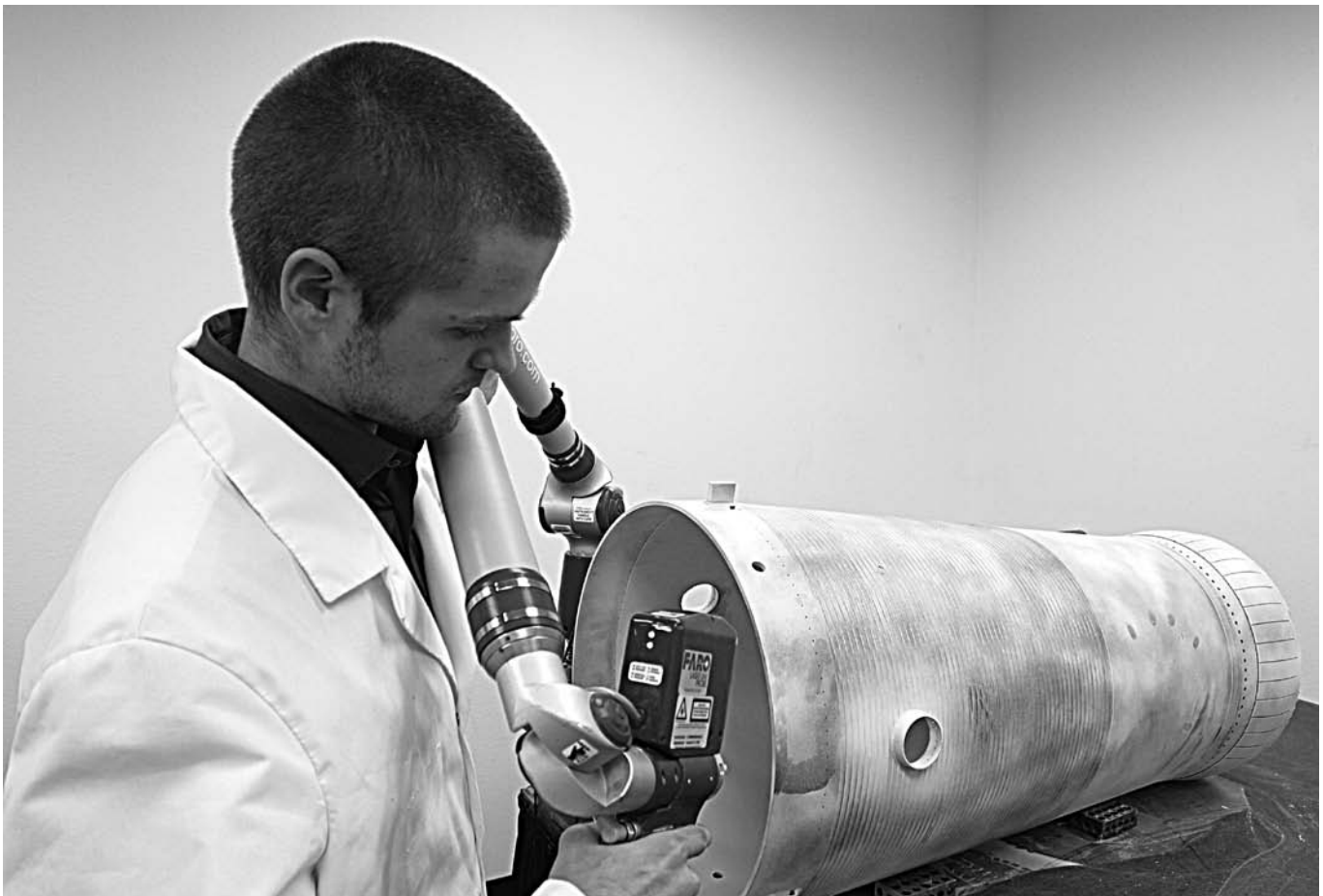
Brian Degraffenreid, Q-Plus inspector, uses a Faro Arm equipped with a laser scan head attachment, to get dimensions on a component used in power generation. Q-Plus also uses the Faro Arm to do on-site work at customer locations.
